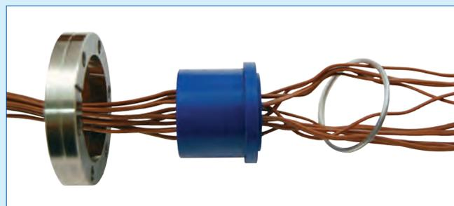
*Figure 2: To control CTE mismatch while maintaining hermetic performance, previous cryogenic feedthroughs encased the conductors in an epoxy slug which would then be compressed between two flanges and a metal gasket.*
