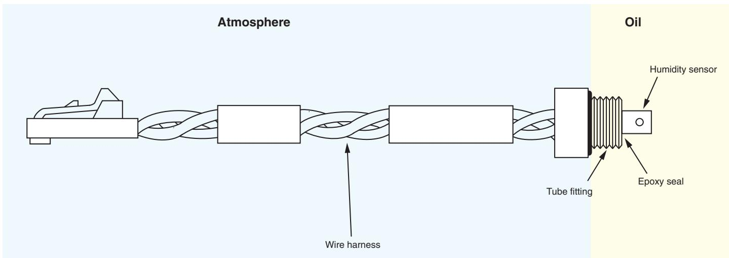
Yet the sealed circuit board proved far easier to design than to manufacture. Stapleton says that early prototypes of the assembly didn't perform well due to a CTE mismatch between the different assembly components. "The CTE mismatch opened up leak paths between the circuit board and epoxy," he explains.
